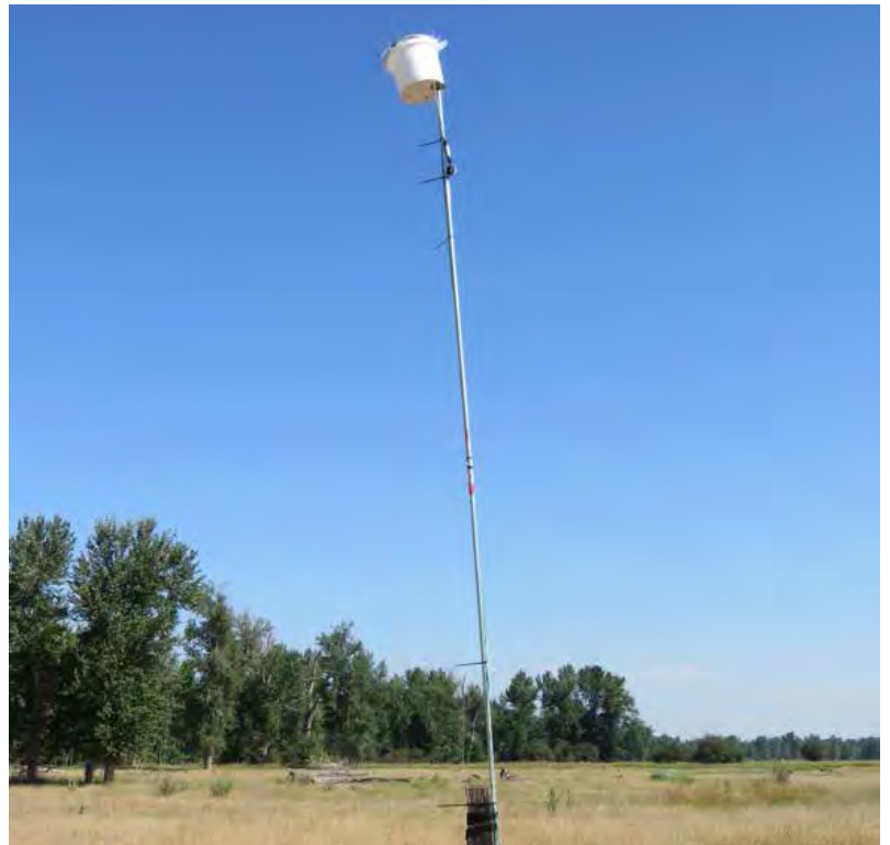
Microphone and mast we installed at Teller. The microphone element is housed in the white bucket.
